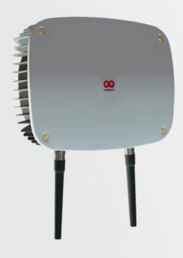
The Wireless Management Node of GlobiLED, referred to as "GlobiNode" (GN), is an outdoor intelligent Gateway, with an integrated webserver, which serves as the connection gateway between the Light Management Software (LMS) and the LED Street Lights. It communicates in real time with the LMS and the Cloud via a 4G or 3G wireless interface (using dedicated APN and Private IP). It is controlled & upgraded remotely via LMS.
